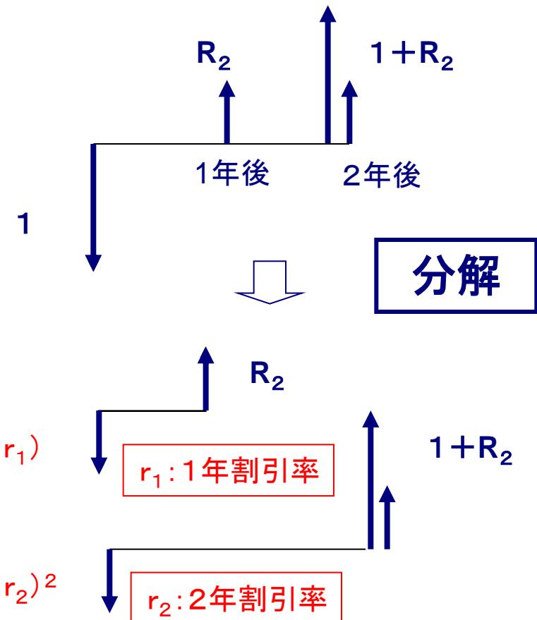
$$1 - R_2 / (1+r_1) = (1+R_2) / (1+r_2)^2$$
